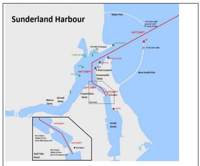
Dock gates are generally opened approximately 2 hours before High Water (HW) until HW at which time either No1 or No3 gates will be closed depending on the next planned operation.
