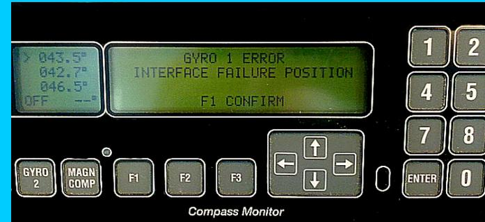
**Gyrocompass: Alarm, and drifts over time**
